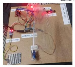
The rain sensor detects rainfall and sends a signal to the Node MCU to activate the servo motor for crop protection. It ensures automatic shielding of crops during rain to prevent water damage
