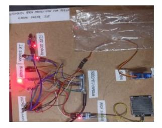
The fire sensor detects the presence of fire in the field and immediately triggers a buzzer alert through the Node MCU. It helps in early fire detection to protect crops from potential damage
